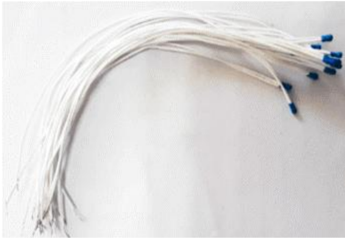
Fig: Temperature sensor
